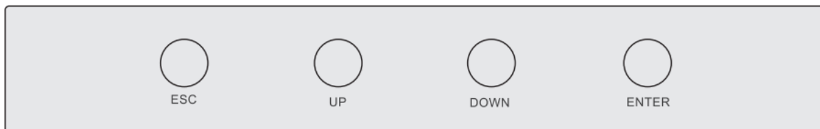
Figure 2.1.4.5 Keypad of Solis inverter
