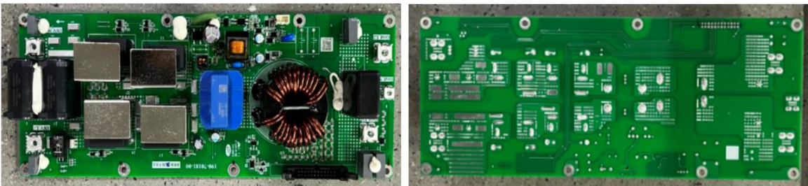
Figure 7 Photo view of Output Board (STL)
