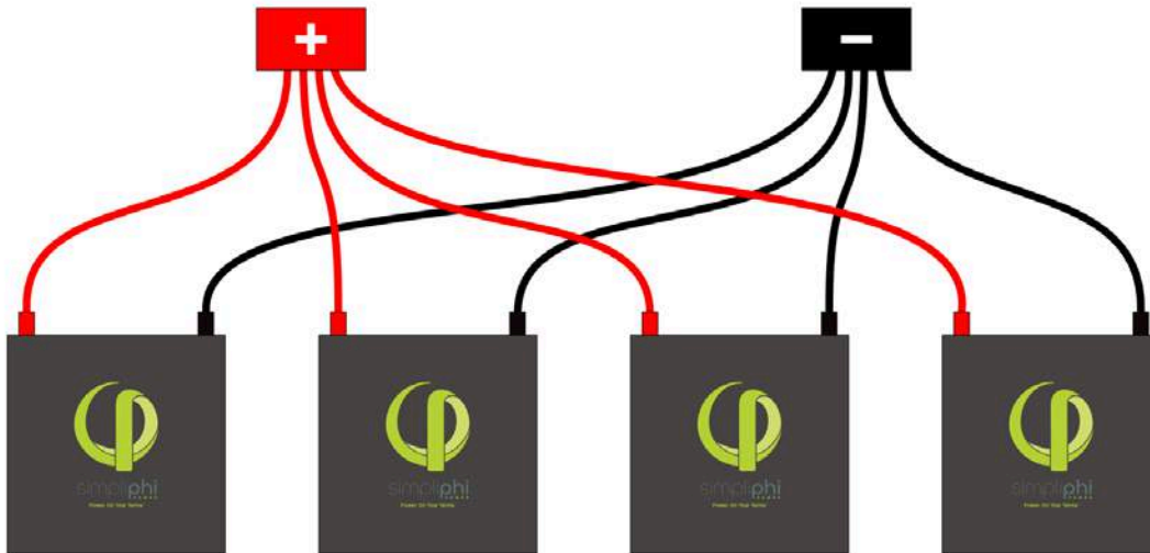
Figure 4.0 - Four PHI 3.5 Batteries in Parallel
